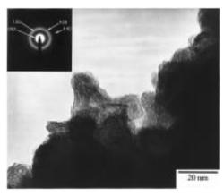
Figure 2. TEM micrographs of sonochemically prepared MoS<sub>2</sub>. Basal planes are seen as dark fringes with interlayer spacings of  $0.62 \pm 0.01$ nm, the same as those for conventional MoS<sub>2</sub>.
