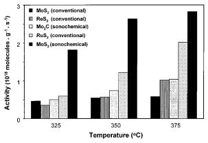
**Figure 3.** Catalytic activities of various catalysts in thiophene HDS as a function of temperature.
