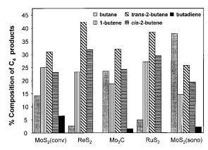
Figure 4. Distribution of C<sub>4</sub> hydrocarbon products observed during thiophene HDS with various catalysts at 375 °C.
