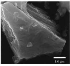
Figure 1. SEM micrographs of (a, top) sonochemical and (b, bottom) conventional preparations of MoS2.
